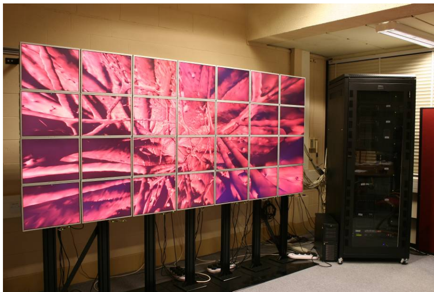
Figure 5 The powerwall displaying the MRI visualization
